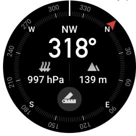
Tap the button on the screen to lock the current 12 o'clock position. Then, when you change the direction, the interface will display the angle between the new 12 o'clock direction and the previous 12 o'clock direction.
